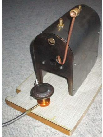
After mounting the various parts on the boiler I filled it with 150ml of water and lit the burner. It took a few minutes before the water started boiling and the pressure rose to 2 bar, and then the safety valves opened and the pressure stayed at 2 bar.
