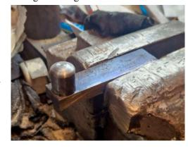
A similar approach was done on the small bushes but I could use a ball peen hammer. I used some packing between the soldering plug and the bush to protect the surface.
