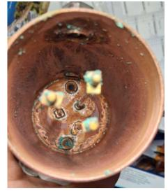
After cleaning the second endplate and stays and nuts were fluxed and some silver solder rod placed around the gaps to be soldered—right photo. When the temperature was high enough more silver soldering rod was applied.
