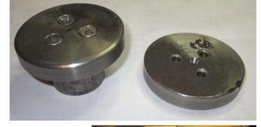
On a piece of cardboard a 24mm dia circle was drawn and three points marked out 120 deg. apart. This was used as a template to drill three 3.3mm holes in the endplate former, the holes were then tapped M4. Three grub screws were inserted in the holes, protruding about 1.5mm.
