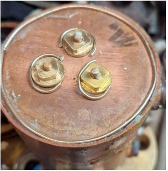
The left photo shows the brazed barrel cooling down. After cooling it was pickled in Citric Acid solution and washed with water.
