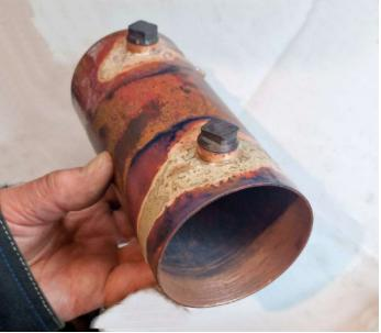
After the first brazing, the inside end of the barrel was cleaned with emery cloth and the already brazed bushes got some new flux. The endplate and stays were fluxed and placed in the hearth and brazed – left photo. The top cover of the hearth has been removed. The second endplate was used to hold the stays in the correct position at the other end of the barrel.
