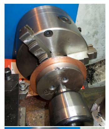
Next, the ball bearing spinning tool was mounted in the tool holder and the first step in forming the endplate started. Then the endplate was removed from the lathe and heated to red with a propane torch to soften the copper. After it cooled, the endplate was mounted in the lathe again and the spinning continued. About four heating – cooling and spinning cycles were necessary to form the endplate. After spinning the endplate was slightly oversize so it was turned on the outside – photo below:
