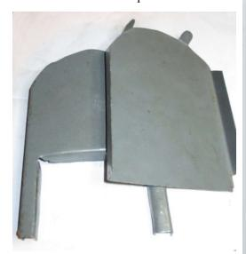
I drilled a few 2.5mm holes and tapped them M3 so it would be possible to clamp the parts together.
