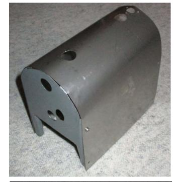
To make stronger threads in the endplates I silver soldered (brazed) some pieces of brass to the rear side of the mounting holes and drilled and tapped M3 again. While the parts cooled after brazing I applied some linseed oil to blacken the endplates and provide some corrosion resistance — right photo. The photo also shows the burner I'm using to heat the water in the boiler.
