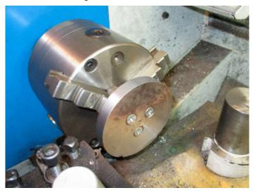
The diameter of the former is the inner diameter of the copper tube minus twice the thickness of the endplates.
