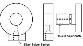
The semi-circular part was milled on a rotary table – right photo. And then silver soldered (brazed) to the siphon.
