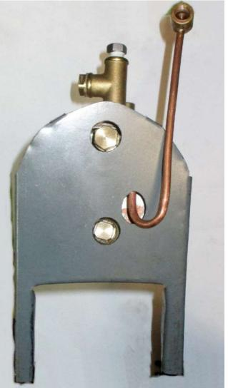
The rest of the boiler cladding was made from stainless steel. I drilled the holes for the two main bushes and a slightly smaller hole for the chimney before bending. This made it difficult getting a smooth curve, I don't know how easy it would have been to drill the holes after bending.
