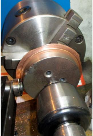
After turning the endplate fitted well into the copper tube – right photo.
