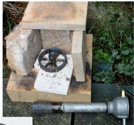
The left photo shows the flywheel so far, after pickling in citric acid solution. The saw cuts at the end makes it easier for my old fingers to screw the spokes into the hub before soldering (using a small screwdriver).
