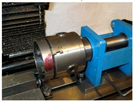
The next job was to drill six 5mm holes 60 Deg. apart in a 20mm dia. mild steel rod to make the hub. The holes were drilled to a depth of just over 5mm. This was done in the indexer almost the same way described before – right photo.
