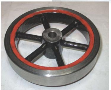
After a bit of elbow grease and emery paper the flywheel was ready for some paint.
