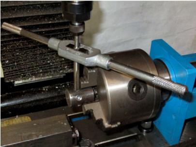
One end of the spokes were threaded M6 using a tailstock die holder, so one end of the spokes can be screwed into the hub, so even if my silver soldering (brazing) isn't entirely successful, the spokes will not come out – right photo.
