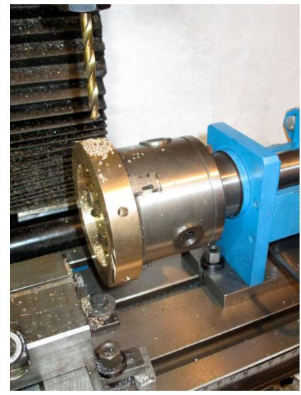
A piece of 20mm dia. brass rod was used for the hub. The indexer was used to drill six 5mm holes (spaced 60 deg. apart) to a depth of just over 5mm. The holes were then tapped M6 – right photo.
