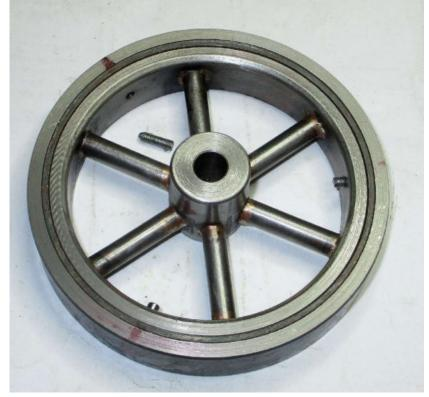
them. After the glue cured the protruding part of the screws were sawn off and then a small file to clean up.
