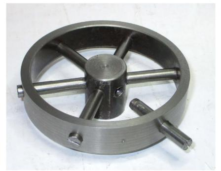
Here are the parts silver soldered (brazed) together in my makeshift hearth. I fluxed both around the hub and the rim and applied the silver soldering rod to the spokes both around the hub and the rim.
