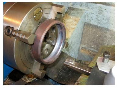
will rest on the little shoulder in the outer rim (tyre) while the glue cures. To the right is a photo of the flywheel before applying any glue. Since the flywheel will be mounted on a mandrel between centres and finish turned in the lathe I wanted to make sure the two parts of the rim didn't move. The three holes in the inner rim that I tapped M3 was used to mark the inside of the outer rim (tyre). I could then use a handheld drill with a 4mm spotting drill to drill three shallow points.
