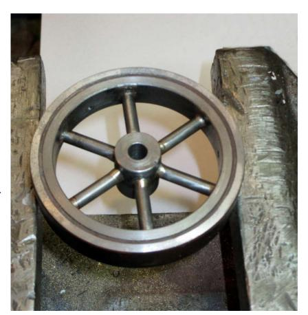
I then made three pointed grub screws (set screws), when they are screwed into the tapped holes in the inner rim and into their shallow points they will secure the two parts – right photo. Felt pen marks were used to show how to orient the two parts.
