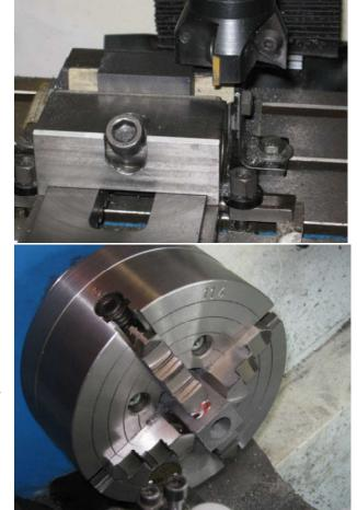
The work was transferred back to the milling machine and the *Valve Pivot Screw* and the four port openings were marked out on the *Port Face* at a PCD of 15mm. I used a 2mm drill for the ports and drilled them to a depth of just over 3mm.
