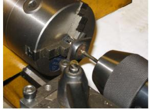
four 3mm holes 90 deg. apart in the Top Cover and used the Top Cover to spot the corresponding holes in the Cylinder top face. The four holes in the Cylinder were drilled 2.5mm and tapped M3.
