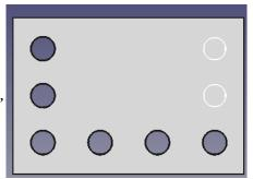
Now select *Hole* in the tasks tab (or click on one of the circles you just made) and create two new *holes* with *Profile* set to *None*, *Diameter* to 15.8 (as you did with the first hole). The hole can be renamed to SecondHole. You can also select the two temporary holes to the left and press the *Delete* button. You may have to click the circle you just made and repeat the *Hole* procedure. Your model should look like this:
