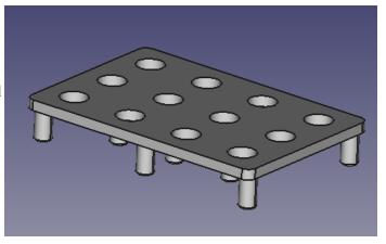
In the Combo **View** Tasks tab click Create Body, Create Sketch and select XY-Plane. Set Grid Size to 10mm and tick Grid Snap and draw a rectangle (Sketch, Sketcher Geometries, Create Rectangle) 148 x 100 mm in size, click Close when finished. If the rectangle doesn't show up on screen click the fit button.
