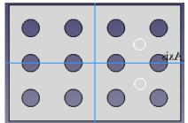
In the *Tasks* tab select *Pad* to extrude to a *length* of 18mm and click *OK*.
