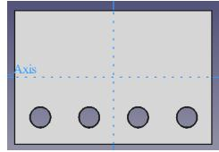
To make it easier to create the other two rows of holes you can use the *LinearPattern* option to create 3 holes in the other direction, just remember to set Direction to *Vertical Sketch axis*, *Length* to 60mm and *Occurrences* to 3. The two new holes will be deleted later, your model should look like this:
