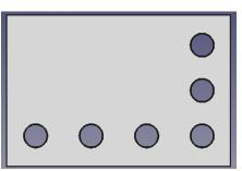
*You can now use the LinearPattern* feature to make the last two rows of holes, click on one of the SecondHole and just remember to tick *Reverse Direction*, *Length* to 110mm and *Occurrences* to 4.
