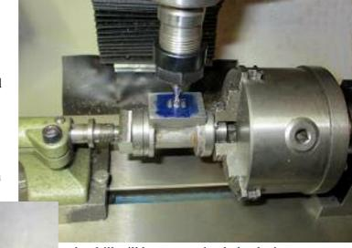
slot drill will have a starting hole, the in ports were milled to a depth of just over 4mm and 5mm wide. I used the same procedure for the exhaust port, except I used a 3mm drill and a larger slot drill.
