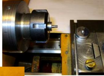
The piston could now be mounted on the mandrel and turned to a sliding fit in the cylinder. I used a parting off tool to turn a
