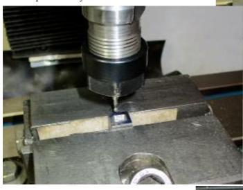
A smaller slot drill was used to mill the cavity to the correct dimensions. It should be nearly as long as the distance between the inside distance between the 1.6mm wide steam in ports, I went for 6.3mm.
