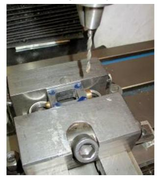
The Steam Chest can then be used to spot the corresponding holes in the Cylinder. The holes
