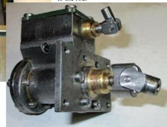
The Crosshead was turned from a Cast Iron rod and the Trunk Guide fabricated from some mild steel
