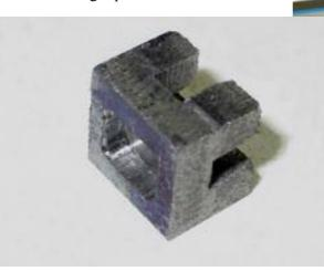
One slot will allow a small nut, the other will allow the Valve Rod to pass. The underside will be rubbed flat on fine emery.
