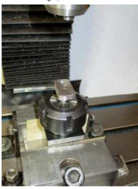
and using the dials on the handwheels I could drill the hole for the crankpin with a 9.5mm offset – see photo above. This will give a throw of 19mm
