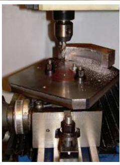
The two pieces of the base was clamped together with M6 bolts and clamped to the Mini-Mill table. A 6-mm pilot hole was drilled through. The first 25-mm was opened up to 16-mm with a twist drill. I then used a boring head to bore the hole to 20-mm diameter to a depth of 25-mm (right picture).
