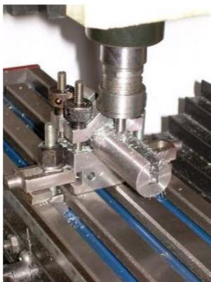
To make the bush with the 6.5-mm square hole I followed Ron's description. This part was turned slightly oversize. Then I mounted the work in a V-block and milled a slot to the required depth with a 6-mm slot drill; the slot was then made slightly wider (6.5-mm) by adjusting the cross feed wheel.
