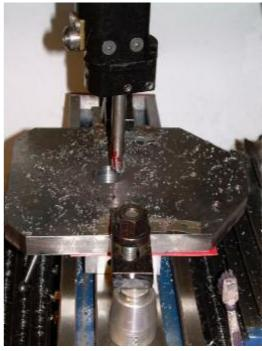
I also drilled four 5-mm holes close to the corners of the base, two of them will be tapped M6 and can be used to clamp the table to the base.
