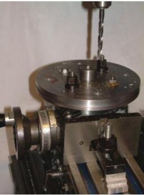
rotary table, I could only mill four of the eight slots at a time. The milling was a slow process, I started with a 6-mm slot drill, then 8-mm milling through the table. Then I used a 13-mm end mill and milled to a depth of a little over 8-mm. This way the slots get a T-slot appearance and will accept suitable T-nuts with the table mounted on the base.
