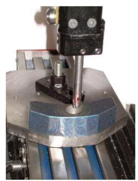
The hole for the table in the base could not be bored in my small lathe, so I clamped the base to the mill table using 1-2-3 blocks to raise the work above the mill table. With a Dial Test Indicator I could centre the Mini-Mill spindle (bottom picture).
