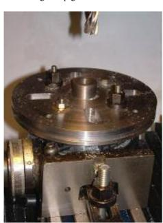
I could now drill four new 6-mm holes rotated 45 degrees from the existing holes (right picture). These holes served as a starting point for four of the eight slots in the table. Since I was using four holes (in slots to be) for clamping the table to the
